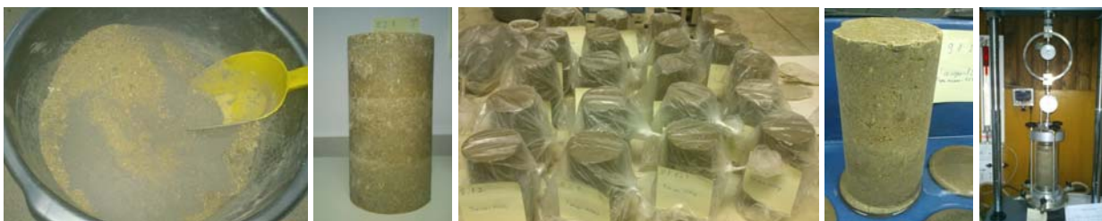
Figure 1. Specimens preparation, curing, soaking and testing
